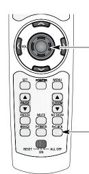
\_PRESENTATION POINTER button Move the pointer on the screen with this button.
